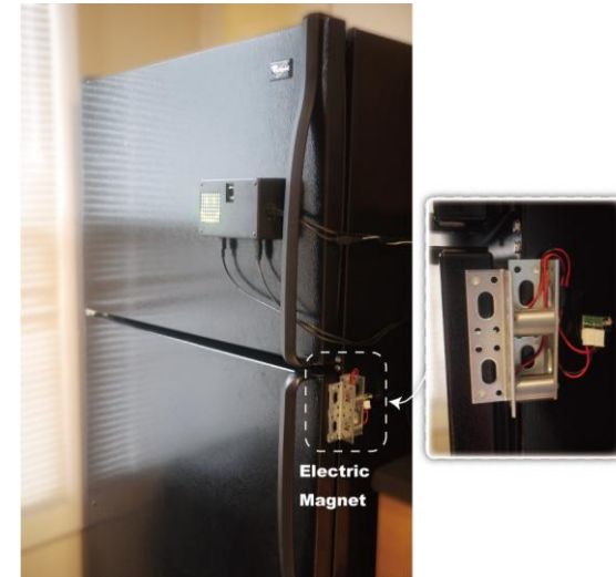
Figure 5. We combined the HappinessCounter Box with an electric magnet and attached it to the refrigerator door.
