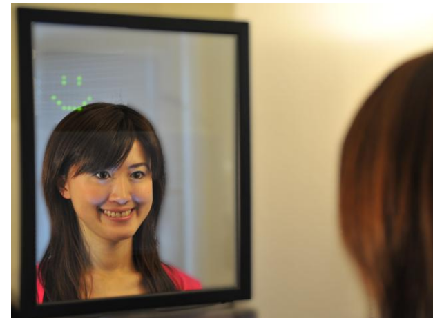
Figure 1. The HappinessCounter encourages users to smile in their daily lives by providing feedback about their smile and combining other reinforcing tools. The system detects a user's smile using the smile-recognition engine, and displays the smile icon as visual feedback in the corner of a mirror.
